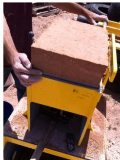
Figure (36) Machines produce single, a few or large number of stabilized earth bricks
