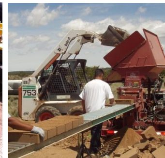
Figure (36) Machines produce single, a few or large number of stabilized earth bricks
