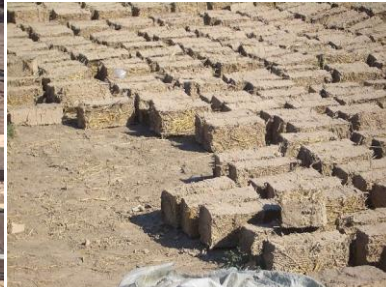
Figure (25) Chopped straw used as stabilizer in some areas as Saudi Arabia
