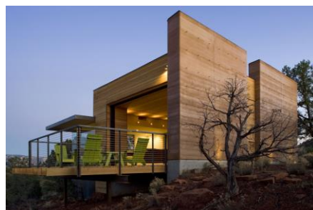
Figure (23) Desert courtyard house, a modern rammed earth project designed by wendell burnette architects
