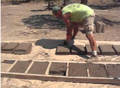
Figure (24) Multi-framed to produce a large number of adobe blocks
